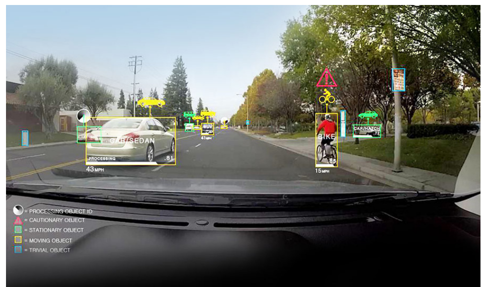
Figure 1 – Object classification using NVIDIA’s Advanced Driver Assistance System (Source: NVIDIA)
